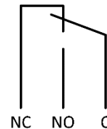
Deactivated relay position
